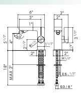
2 ways out thermostatic concealed mixer, with one handle for temperature control and one handle diverter with flow regulator with stop. 3/4" inlets with adapter to 1/2". 1/2" outlets.
